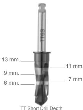
The drill lengths are overestimated by 0.5 mm. compared to the endosseous length of the implants.
